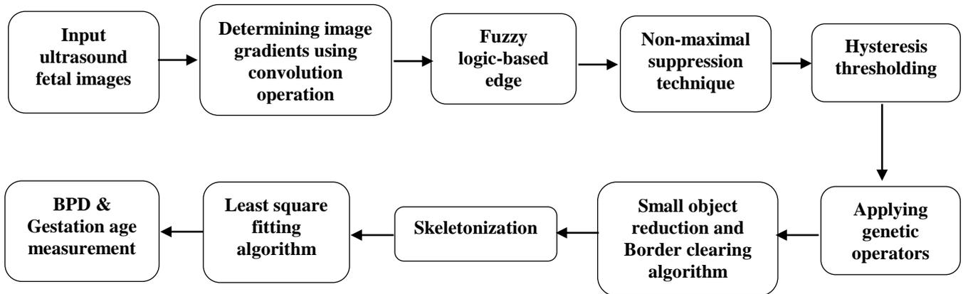
Figure 2: Schematic flow of proposed method to determine gestation age-Step by step procedure
