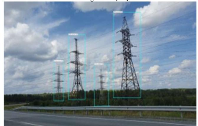
**Figure 7:** Shows power transmission line detection and localization from UAV using DNN [29]
