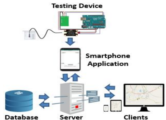
Figure 1: The proposed data flow diagram using testing device, smartphone application, server, database and clients (users).
