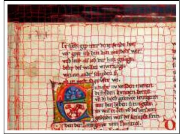
Figure 1: Result from using superpixel method (image from K. Chen et al. 2016).
