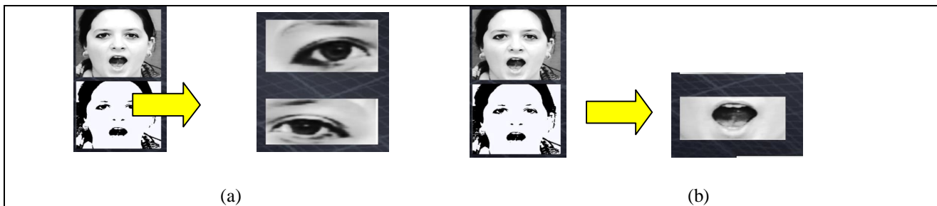
Figure 4: Eyes (a) and mouth (b) region box that being cropped from the face area
