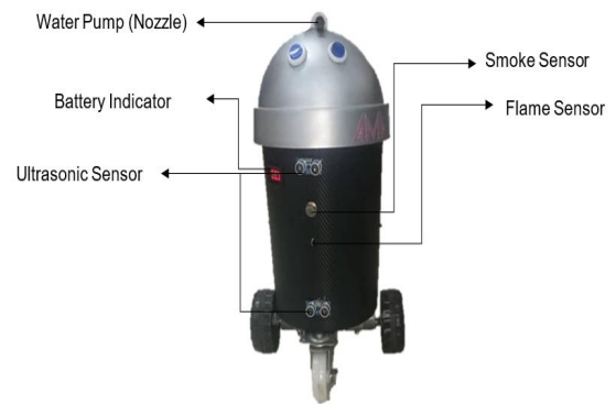
Figure 5a. The final design output of the automated hazardous gas detecting robot (front view)
