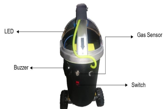
Figure 5b. The final design output of the automated hazardous gas detecting robot (rear view)
