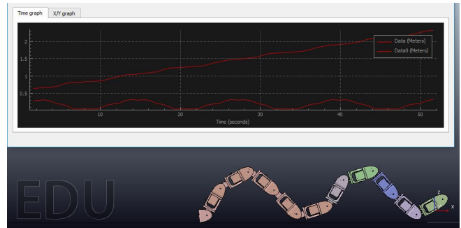
Figure 16: 0.5-D convex configuration produce X-movement 1 m in 30 sec or V=0.0333\text{m/s} with \omega=0.5\text{rad/sec} where V_t=0.0386\text{m/s}
