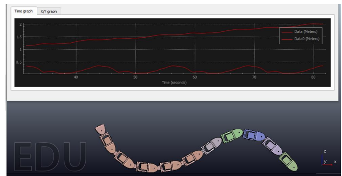
Figure 14: 1-D convex configuration produce X-movement 0.5 m in 34 sec or V=0.0147m/s with w=0.5rad/sec where V_{theory}=0.0123m/s
