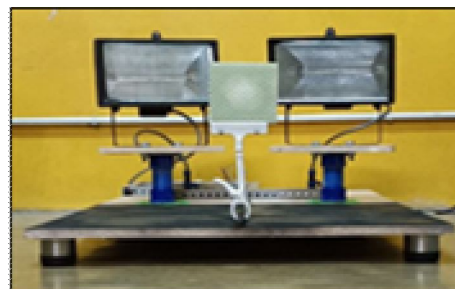
Figure 3: Front view of thermography setup
