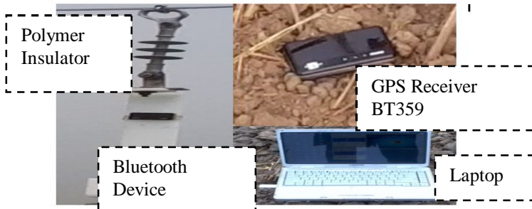
Figure 1: Main components of GPS based overhead conductor sag measuring system
