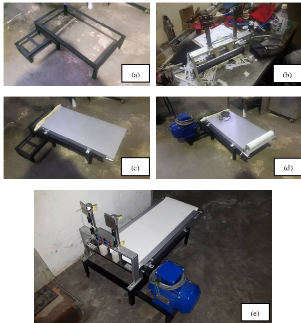
Figure 3: Fabrication process (a) Basement (b) Assembled cutter (c) Embedded supporting frame for the conveyor (d) Tested induction motor and prime roller (e) Attached cutter to the basement
