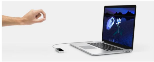
Figure 1: Use of Leap Motion. Leap Motion controller is the object in the center. It is connected to the system on the right side. Hand's interaction with the virtual object is tracked with the Leap motion.
