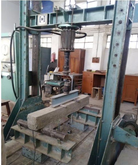
Figure 6. Test setup for four point loading
