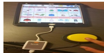
Figure 2: Switch Access Scanning Assistive Technology
