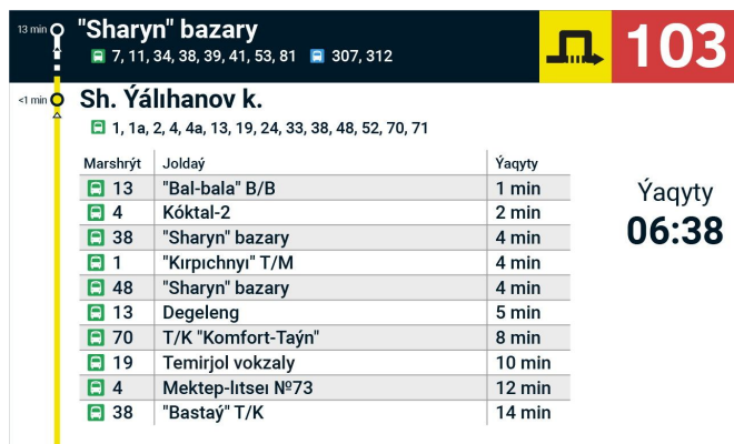
Figure 18: Proposal of the information panel inside of a bus – example for right before arriving to the final stop (display for stop that is a part of operational restriction). Note the diversion symbol and yellow stop marking to alert passengers on the restriction. Express bus line no. 103
