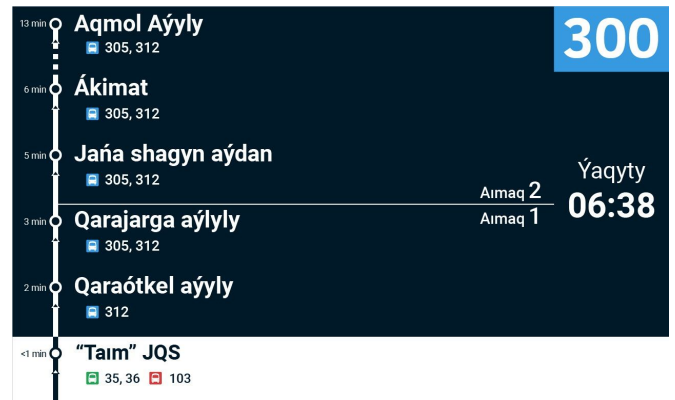
Figure 10: Proposal of the information panel inside of a bus – example for section with 2 different zones. Notice the horizontal line. Suburban bus line no. 300
