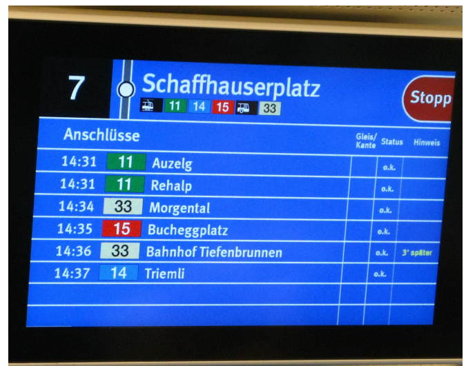
Figure 16: The content of the information panel inside of a public transport vehicle in Zürich (Switzerland) – example right before arriving to the stop
