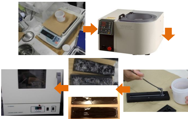
Figure 3: Rubber fabrication process
