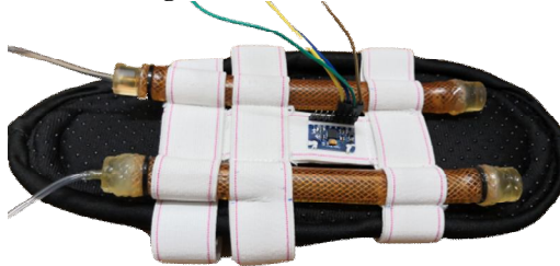
Figure 8: Experimental setup of foot exoskeleton without load (foot)
