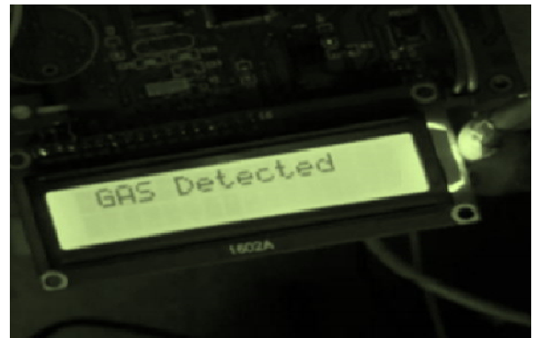
Figure 6: LCD Displays when harmful gas detected
