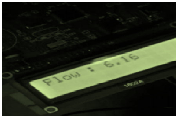
Figure 5: Water flow level displayed on LCD Screen
