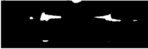
Figure 9: Output Result for AND of RGB and HSV Based from the size of the detected taillights (as blobs), the distance is determined and related to the necessary Pulse Width Modulation (PWM) duty cycle that the PID controller needs to output. The relationship between the PWM duty cycle and the pixel distance of the taillights and the actual distance from the taillights is found to be nonlinear, i.e., hyperbolic and is shown in Figure 10. In order to avoid complex and nonlinear calculations, this hyperbolic relationship is translated into a linear equation by utilizing the inverse of the PWM duty cycle, as shown in Figure 11.
