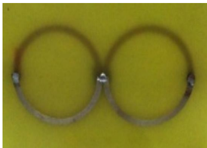
Figure 2: Bi-circular antenna fabrication results
