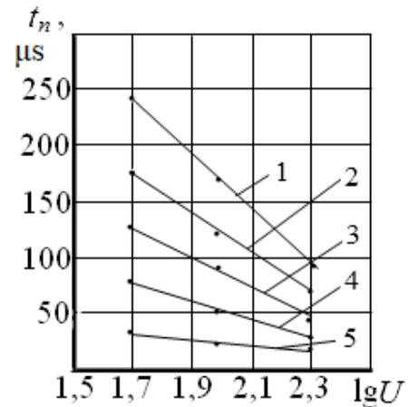
Figure 3: Dependence of the total plasma decay time on  $\lg U$  at a discharge current of 1 A:  $d = 16 \text{ mm}$ ;  $d = 14 \text{ mm}$ ;  $d = 12 \text{ mm}$ ;  $d = 10$ ;  $d = 8 \text{ mm}$
