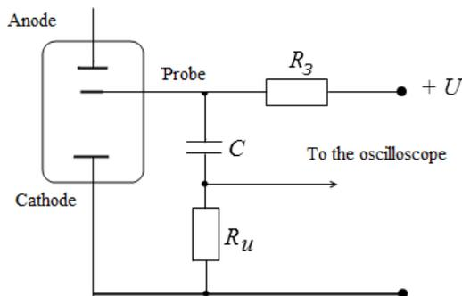
Figure 2: Diagram of probe measurements with storage capacity
