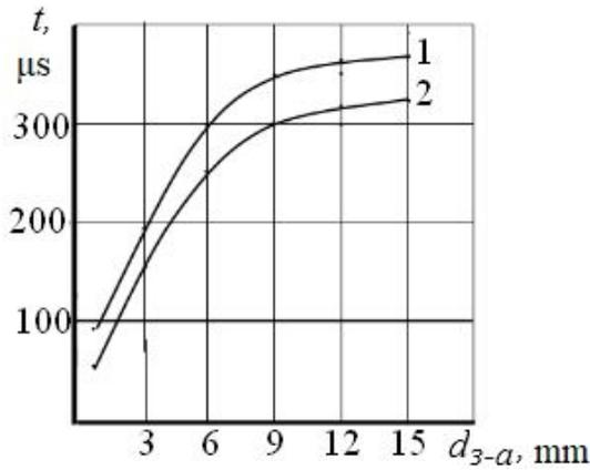
**Figure 4:** Dependence of the plasma decay time between the cathode and the anode at a pressure of 0.2 mm Hg, with a reverse voltage  $U = 100$  V for various values of the discharge current: 1 -  $I = 5$  A; 2 -  $I = 1$  A
