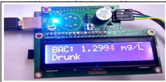
Figure 5: LCD screen indicating that the biker is drunk
