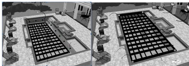
Figure. 2. Proposed Swimming pool with switches arranged all places on bottom elevator –a)lowered – b)raised position.
