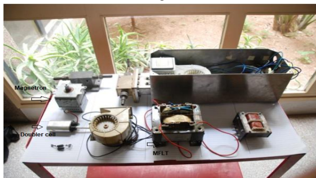
Figure 10: Experimental arrangement for the testing of microwave oven.
