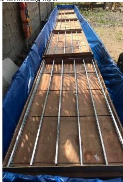
**Figure 4:** Formworks for Wall Panel Specimens
