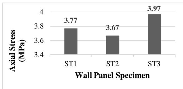
Figure 7: Capacity of Wall Panel Specimen against Axial Stress
