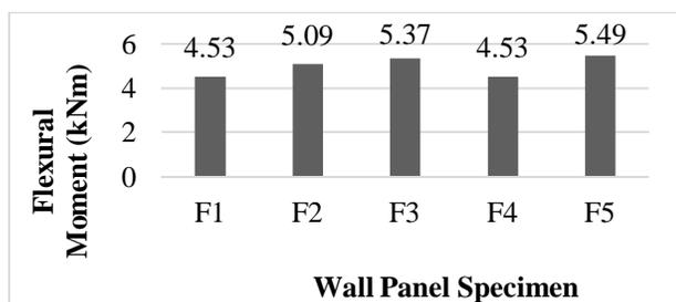
Figure 9: Capacity of Wall Panel Specimen against Flexural Load
