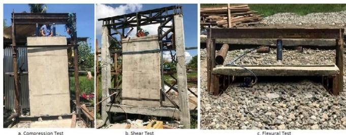
Figure 5: strength Tests for the specimen
