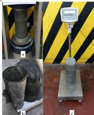
**Figure 2:** Compression Test; b.) Slump Test; and c.) Unit Weight Test of Concrete
