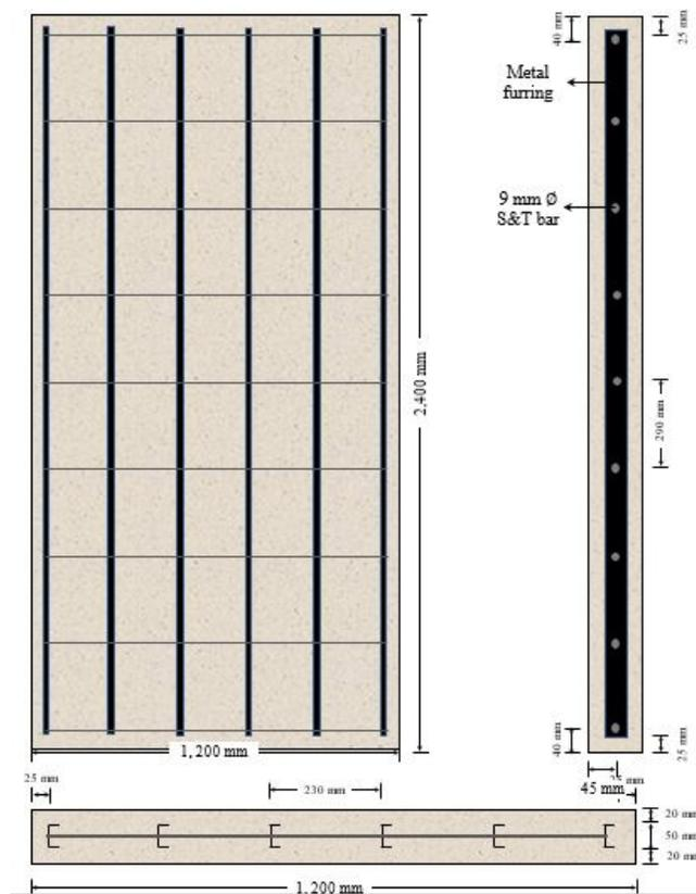
**Figure 3:** 2D Visualization of Wall Panel Design
