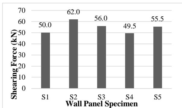
Figure 8: Capacity of Wall Panel Specimen against Shear Load
