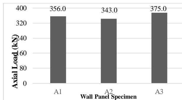
**Figure 6:** Capacity of Wall Panel Specimen against Axial Load
