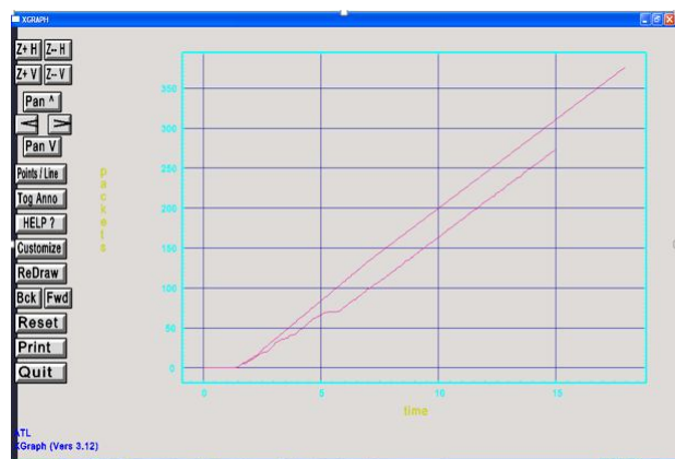
Figure 6: Comparison of Packet Received of 100 Nodes with Basic DSR and Enhance DSR
