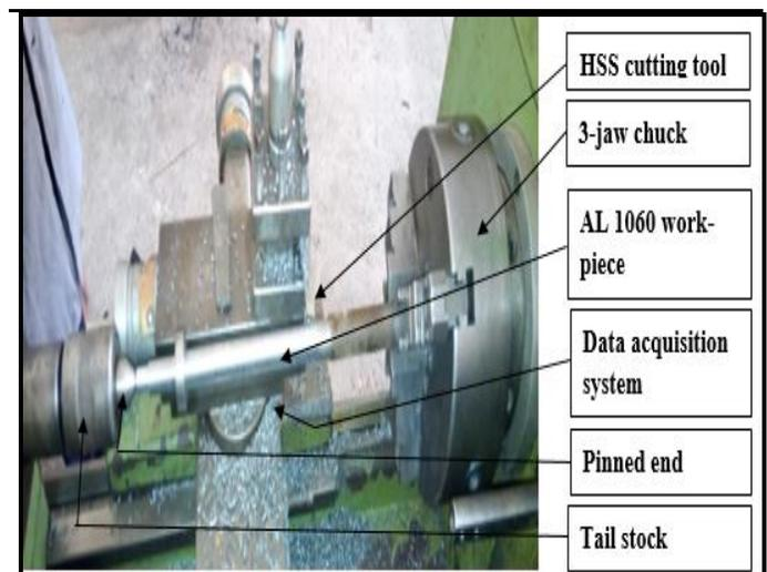
**Figure 1:** The Experimental Set-Up for the Turning of AL1060 Alloy.
