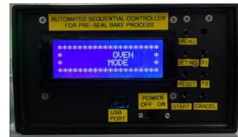
Figure 10: Actual prototype of the automated sequential controller for pre-seal bake process
