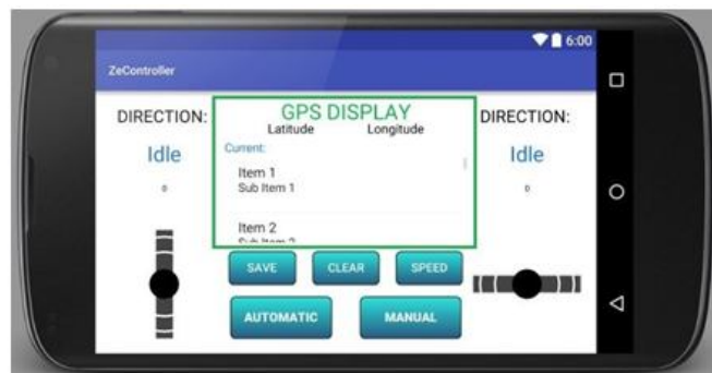
Figure 6: User Interface of the Android-based Robot Controller
