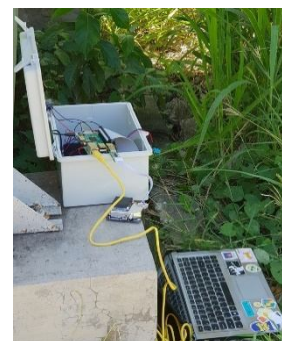
(b) Calibration setup beside the air pollution monitoring station
