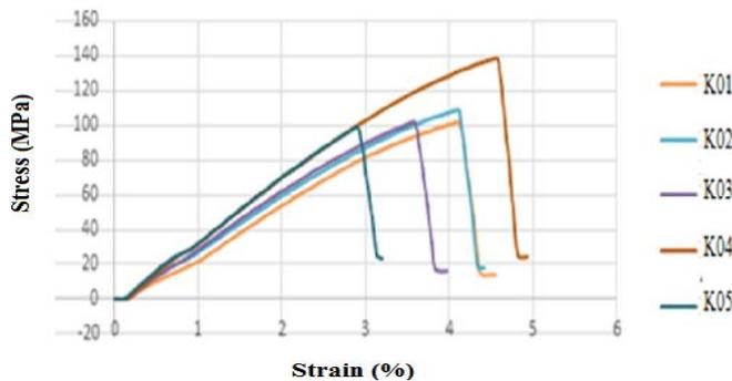
Figure 2: Tensile curves at 0° [2]
