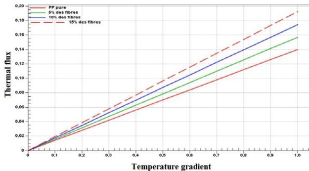
Figure 19: Thermal flux for different percentages of fibers
