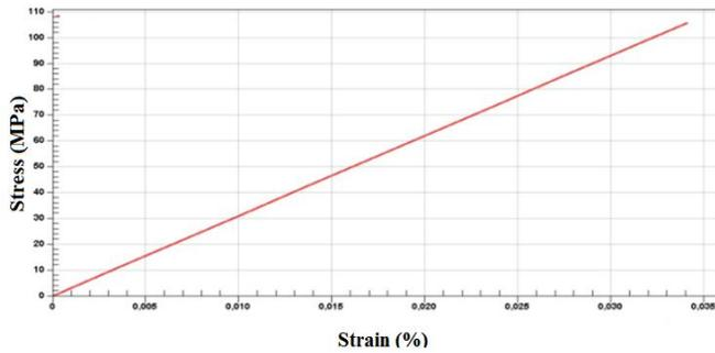
Figure 13: Stress-strain curves at 0° of fiber direction
