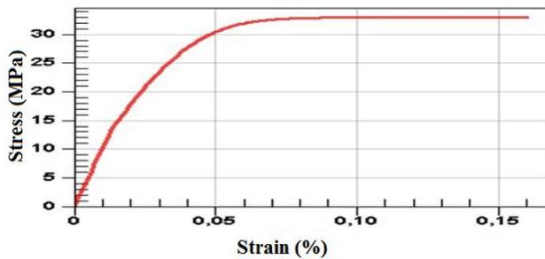
**Figure 6:** Stress-strain curve of the Polypropylene
