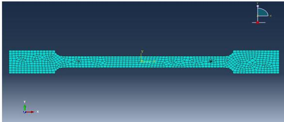
**Figure 5:** Mesh of the specimen
