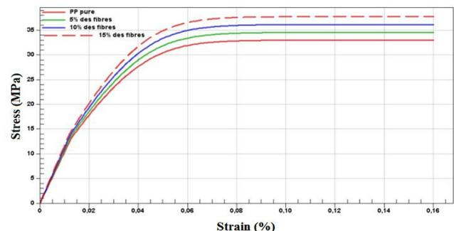
Figure 16: Stress-strain curves of the bio composite
