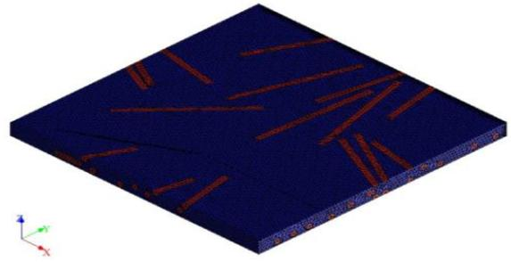
Figure 11: Mesh of the bio composite
