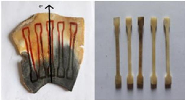
Figure 1: Cutting specimens parallel to the fibers [2]
