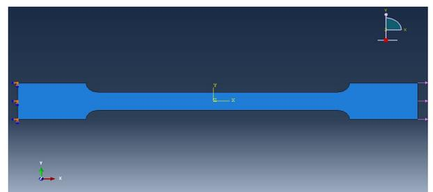
Figure 4: Boundary conditions and loading.
