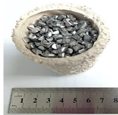
Figure 1: Ceramic mould filled with Al granules before heating.
