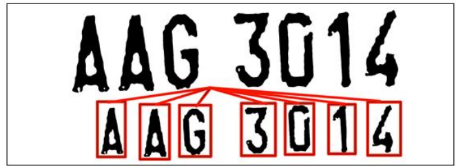
Figure 7: Image Segmentation of plate number
