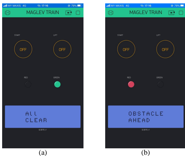
Figure 6: Blynk Interface (a) No Obstacles (b) Obstacle Detected
