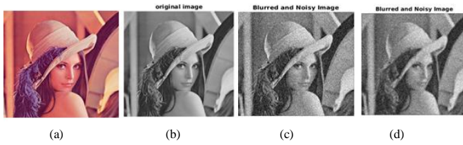
Figure 5: (a) Original color image (b) original gray scale image (c) image with blur and noise in iteration 1 (d) image with more blur and noise in iteration 2
