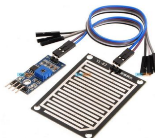
Figure 3: Rain Detection Sensor
