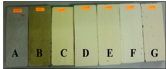
Figure 1: Surface samples for outdoor exposure coated sustainable polymer composites
