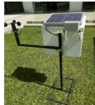
Figure 6: Transmitter Side of the Weather Station
