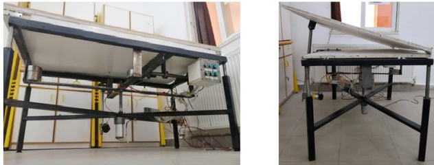
Figure 8: The Manufactured Ergonomic-Automated Adjustable Drafting Table
