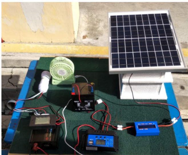
Figure 7: Developed PV training kit
