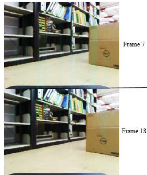
Figure 8: An example of loop closure detected on Frame 18 that matches Frame 7. The threshold number of visual features is set at 8 for accepting a loop closure hypothesis. The green lines show matched features and are more than 8, thus the hypothesis is accepted.
