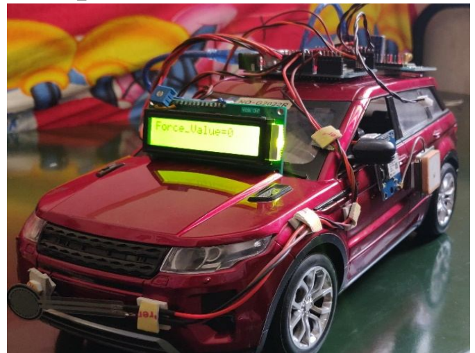
Figure 4 Prototype of the Accident Detection System in Car
