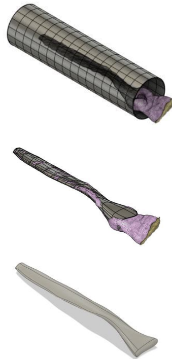
Figure 8: T-spline modeling of a propeller blade from coarse photogrammetry mesh
