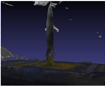
Figure 7: Successful photogrammetry reconstruction of a propeller blade due to applied tack
