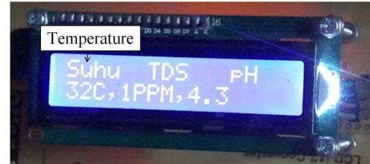
Figure 6: LCD Displaying All Three Measured Variables at the Same Time
