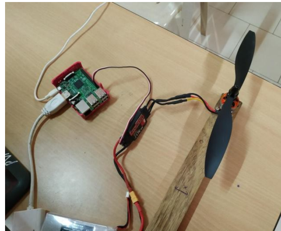
Figure 5: Testing whether brushless motor is rotating or not
