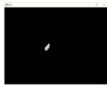
Figure 5: Masked Image Converted to grayscale using cv2.COLOR_BGR2GRAY
