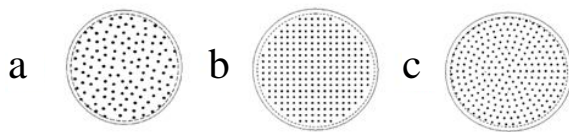
Figure 1: Arrangement of piezoelectric elements in different arrays: (a) – in a random order, (b, c) – arrays ordered in different ways.
