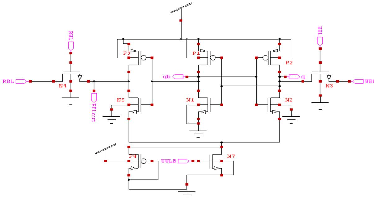
**Figure 4:** Proposed Circuit architecture of 8T SRAM with Virtual ground
