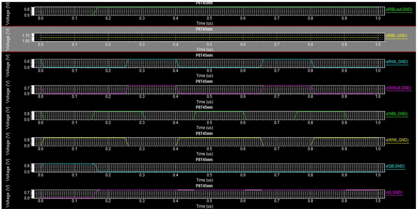
**Figure 6:** Transient results of proposed 8T SRAM Cell
