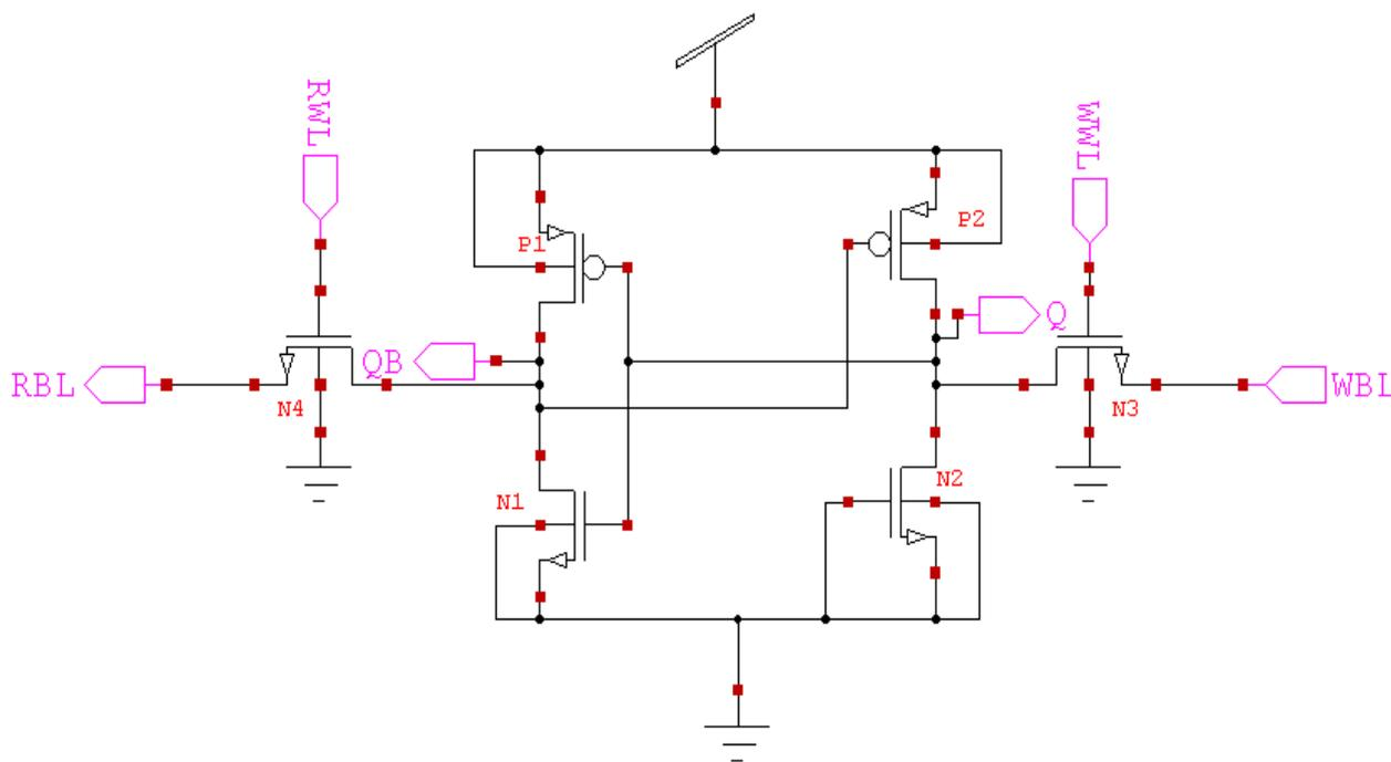
**Figure 5:** Proposed architecture of Single Ended 6T SRAM Cell
