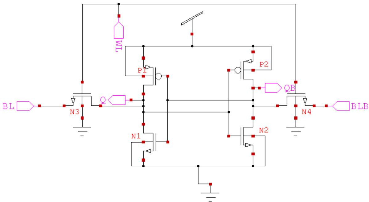
**Figure 1:** Schematic circuit of Conventional 6T SRAM
