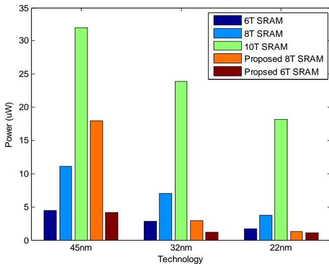
Figure 8 : Power dissipation comparison
