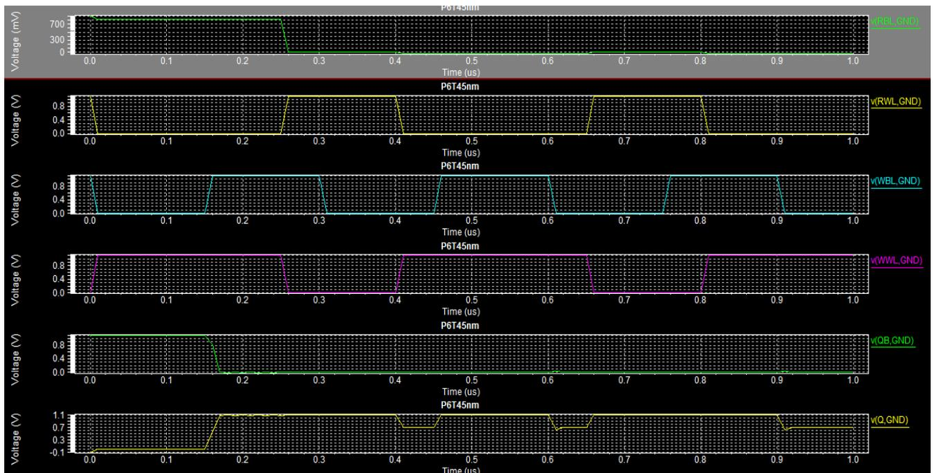
**Figure 7:** Transient results of proposed 6T SRAM Cell
