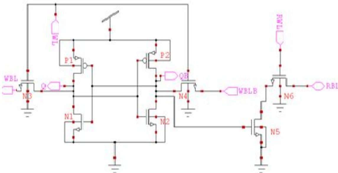
**Figure 2:** Schematic circuit of Conventional 8T SRAM with Dual Port
