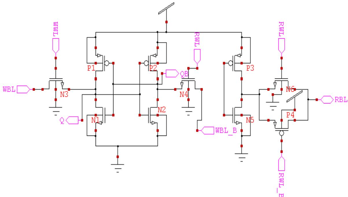
**Figure 3:** Schematic Circuit of Conventional 10T SRAM cell
