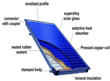
Figure 2: Principal Diagram of a Flat Solar Collector
