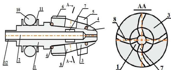
**Figure 1:** Structural diagram of a device for cleaning the inner surface of pipelines
