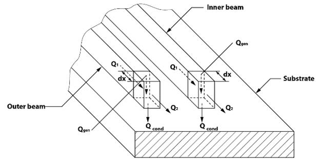
**Figure 4:** Heat transfer paths involved in an infinitesimal element of an electrothermal actuator.
