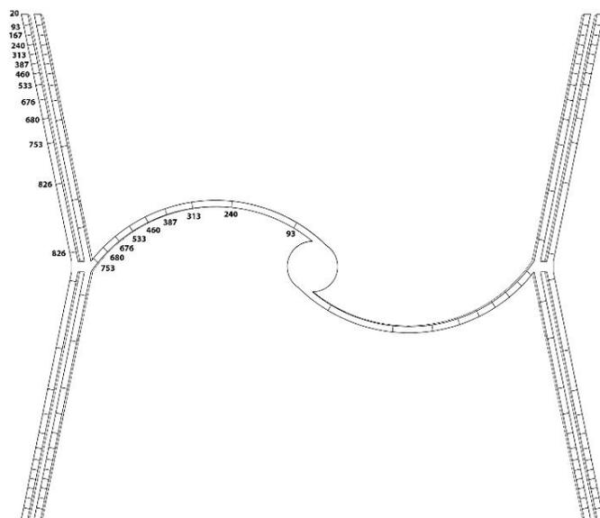
Figure 7: Temperature distribution of the motion converter.
