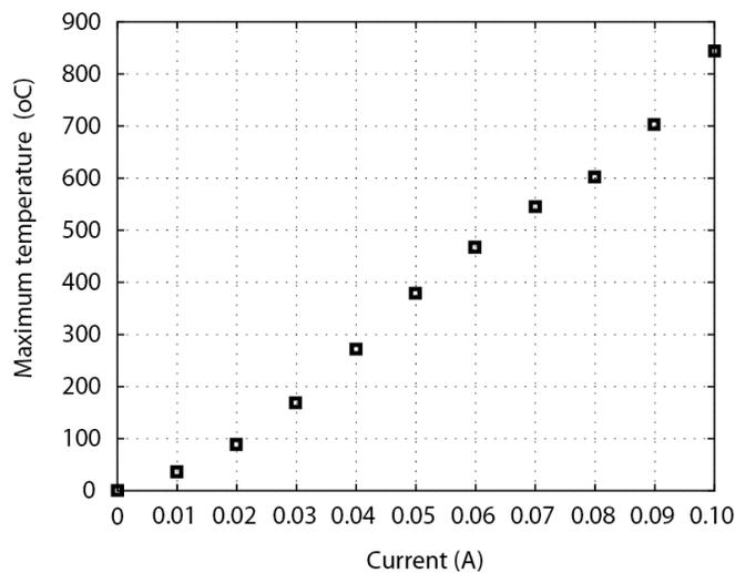
Figure 6: Maximum temperature versus driving current.
