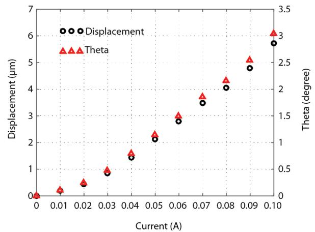
Figure 8: Maximum rotation angle and maximum displacement versus driving current.
