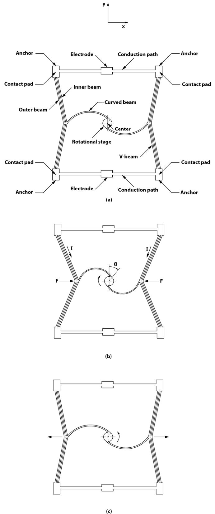
**Figure 1:** Model of compliant bistable mechanism.
