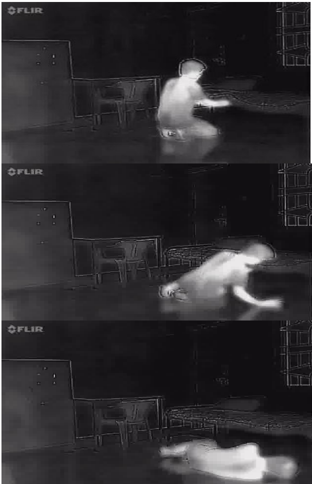
Figure 3: Thermal dataset – ADL and fall frames.
